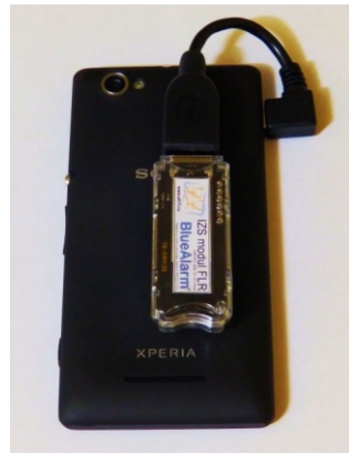
fig. 26 - cell phone with FLR receiver
