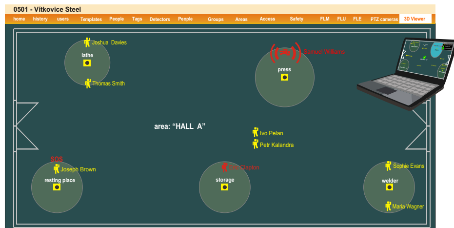
fig. 1 - Ground plan disposition of presence detection and detection of hazardous conditions of people online in the industrial hall
