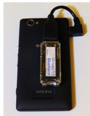
fig. D - a phone with FLR receiver
